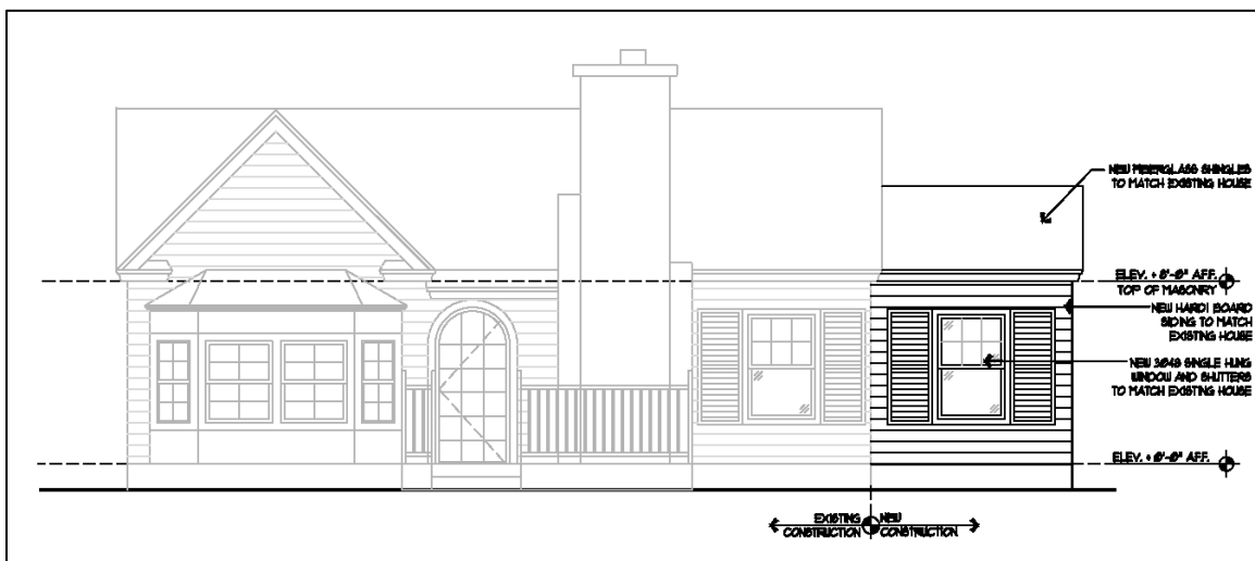
Figure 2: Approved front elevation with new side addition. The plans state that the roofing material will be shingles to match existing house.
